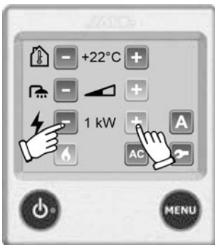
Fig. 163: Heating with electricity
