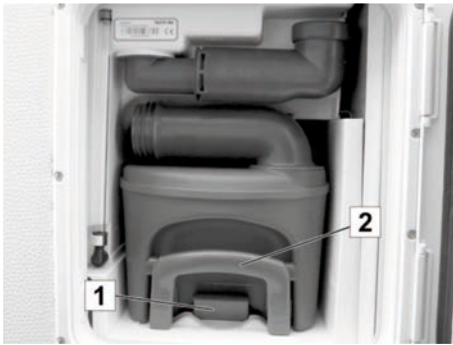
Fig. 192: Waste holding tank in the disposal shaft
