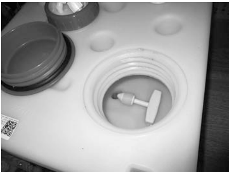
Fig. 102: Drain plug in the fresh water tank
