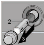
Fig. 214: Changing the batteries of the battery igniter (only if present)
