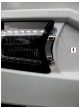
Fig. 226: Reattaching the rear lamp assembly
