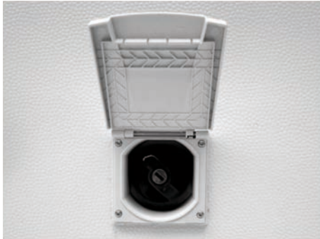
Fig. 88: Fresh water intake port
