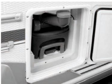
Fig. 47: Holding tank with flushing water intake port
