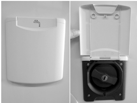
Fig. 22: Fresh water intake port
