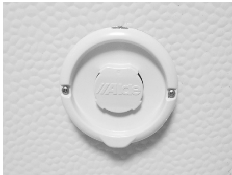
Fig. 82: Wall exhaust stack
