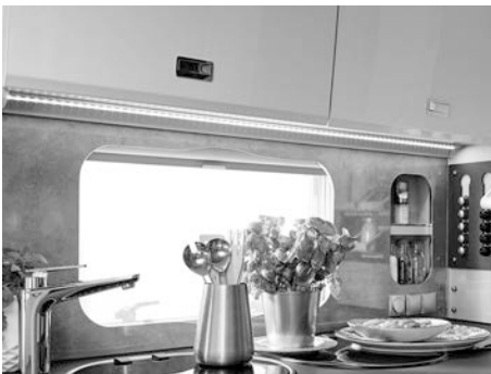
Fig. 64: LED light rail (typical)
