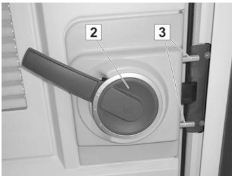
Fig. 17: Door closed and secured
