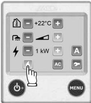
Fig. 162: Heating with gas
