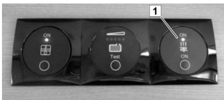
Fig. 130: On-Off switch of the floor heating system
