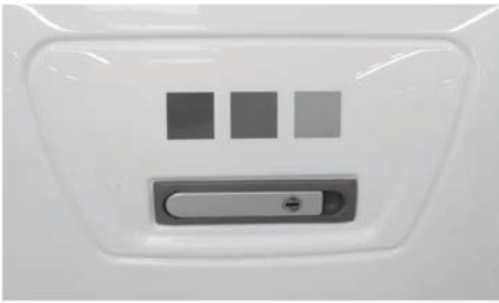
Fig. 69: Gas bottle locker, sealed
