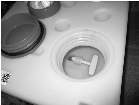
Fig. 103: Drain plug in the fresh water tank
