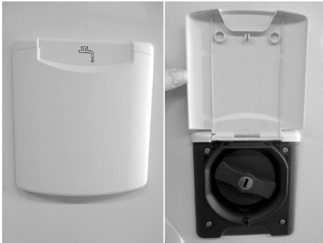
Fig. 100: Fresh water intake port
