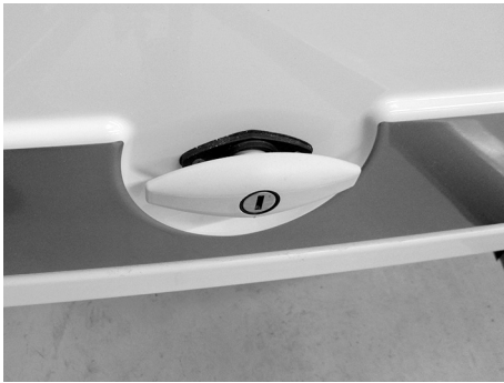
Fig. 31: Gas locker lock
