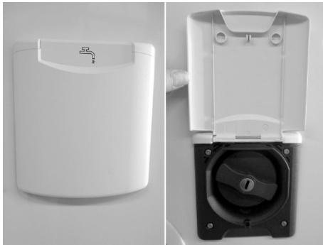
Fig. 32: Fresh water intake port
