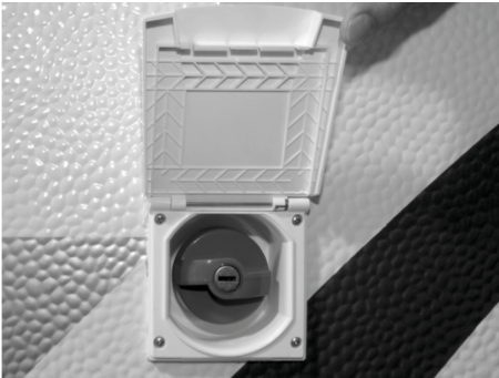
Fig. 91: Fresh water intake port
