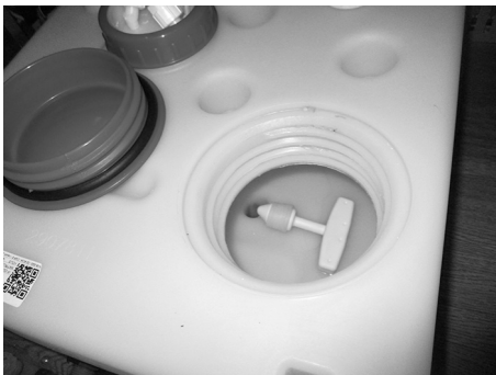
Fig. 95: Drain plug in the fresh water tank
