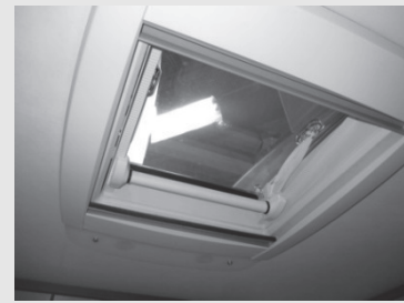
Afb. 33: Dakluik 400x400 mm VisionStar 700x500 mm
